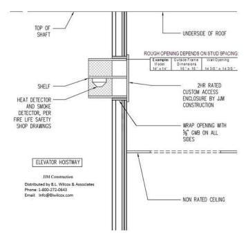
JJM Fire Rated Access Enclosures for smoke detector installation in elevator hoistways provides and approved method that allows for secure smoke detector installation in restricted areas such as elevator hoistways and machine rooms while being serviceable from outside.
